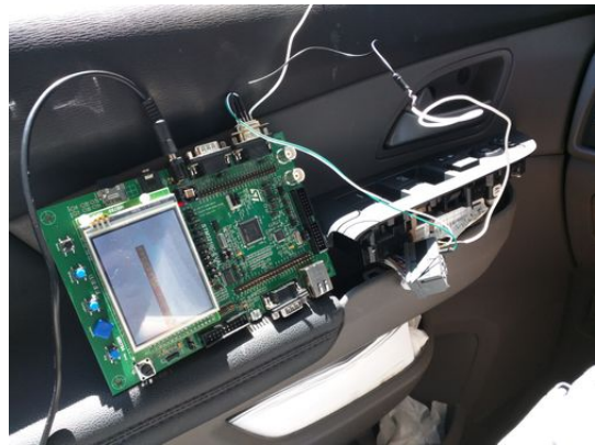
Figure 8: RV-ECU development prototype connected to the body CAN bus of a 2012 Honda Odyssey
